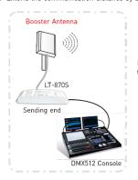
Booster Antenna [Attn] Please install the LED Strip booster antenna LT-874S-5A in high open place, the communication distance can up to Receiving end 1000-2000 meters generally. Booster Antenna LED Strip LT-874S-5A
